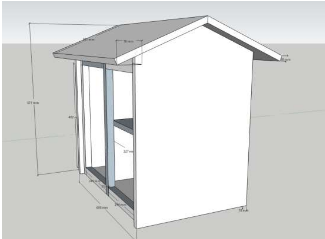
Side on (roof overhang) with dimensions (no doors in this view, just 25mm hardwood waterbar frame)
