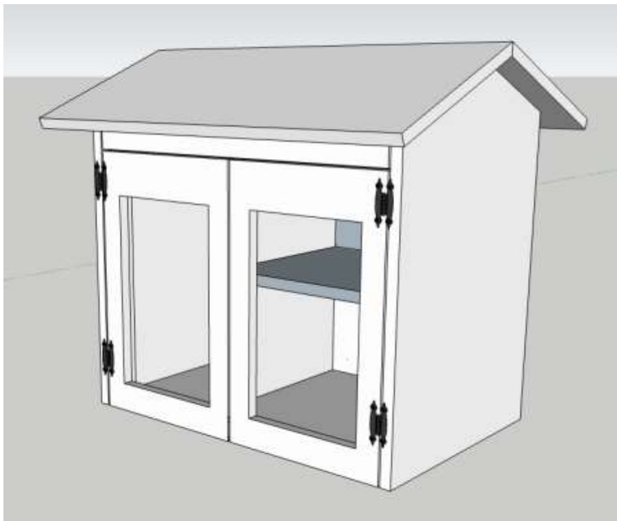
Doors visible with hinges (no Perspex in model but cut out visible for where it'll sit - handles to go on too)
